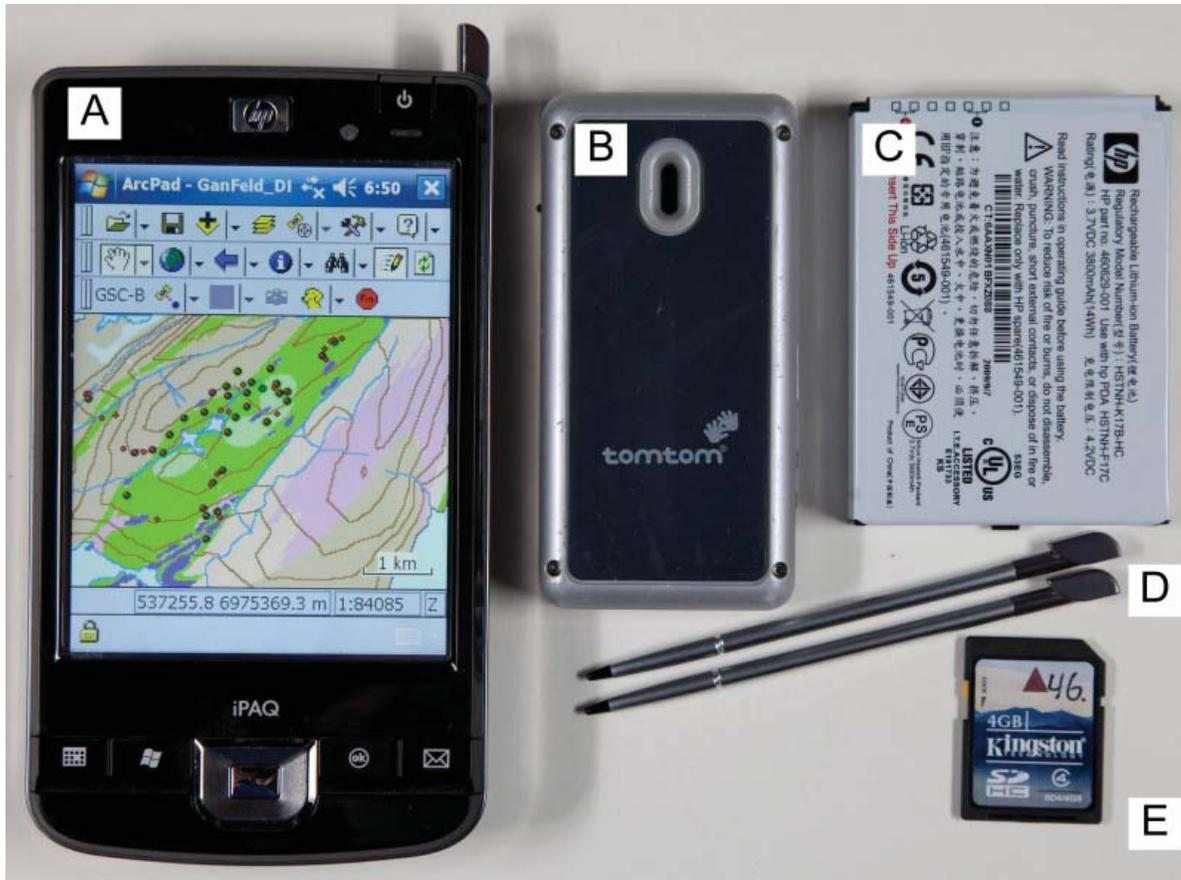
Figure 1. The digital field data capture system consists of: a) HP iPAQ PDA (310 €); b) wireless GPS receiver (48 €); c) HP extended battery (59 €); d) PDA stylus (7 € for each stylus); e) secure digital (SD) memory card (15 €).
