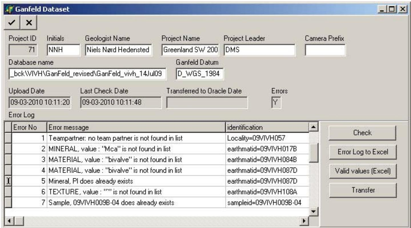
Figure 7. A software routine cross checks the field data with the database and detects inaccuracies which are then listed in an error report. This list helps the geologist to revise and edit the field data.
