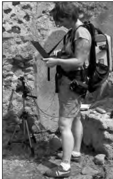
Fig. 2. Hand-held configuration of the FieldSpec®3. with the author taking a reference measurement.
