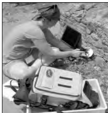
Fig. 3. Tripod configuration of the FieldSpec 3® with the author taking a target sample reading.
