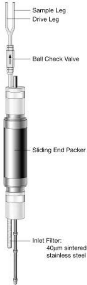
Fig. 1. Schematic layout of the downhole equipment for deploying a U-tube geochemical sampler.
