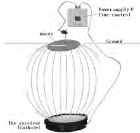
Fig.4. "Dipole CHIM" with time controller
