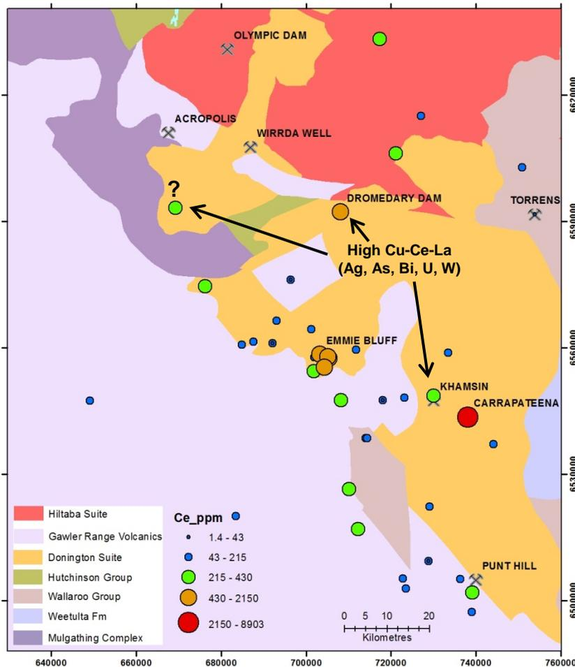
**Figure 6. Ce values from base of cover sampling in the central eastern Gawler Craton, South Australia on a solid geology base map. High Ce values in combination with high Cu and La values can be used to identify proximal mineralisation within basement.**
