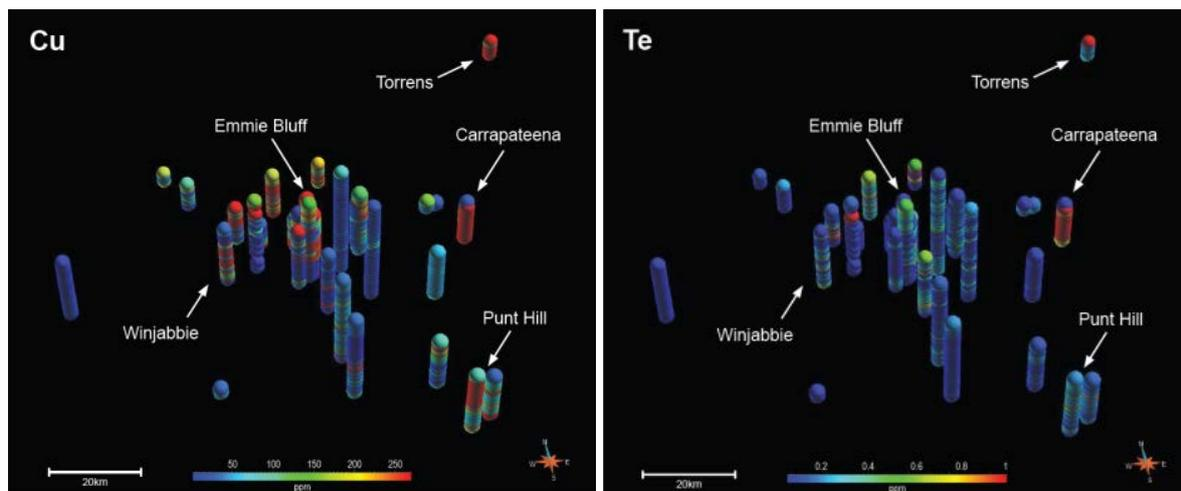
**Figure 5. 3D perspective view of Cu and Te values from down hole samples, central eastern Gawler Craton, South Australia.** Significant mineral occurrences are labelled. High Te values are only associated with ore grade intersections.
