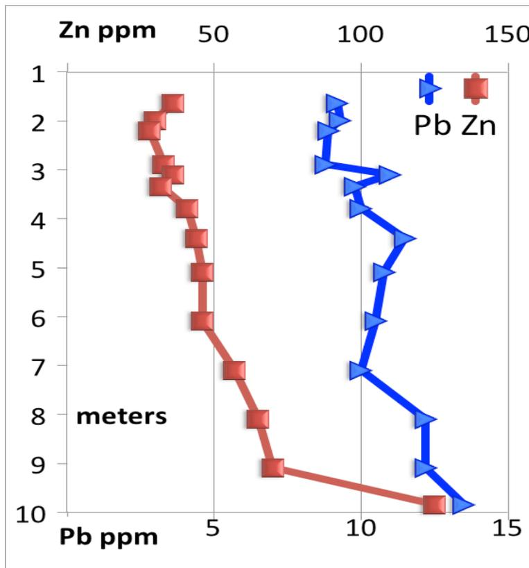
Figure 6. Profile for Zn and Pb in the pit wall from below the calcrete to the unconformity. Ore grade mineralization is not present at the base of this pit.
