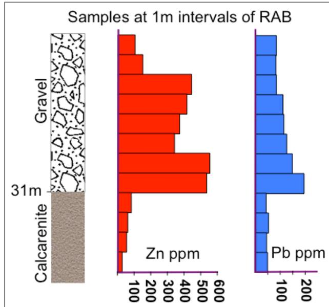
**Figure 7. Example data from the regional RAB drilling program. Following initial screening by FP-XRF highlighting anomalous Zn and Pb values immediately above the unconformity contact. The final 2m samples would be composited and submitted for multi-element analysis. Modified from Schaefer (2008)**
