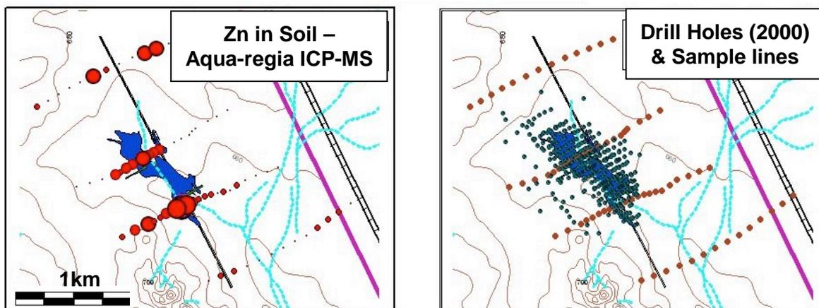
**Figure 2. a- Zn results in soil by aqua-regia ICP-MS.** Symbols are scaled from small Zn (30ppm) to large (65ppm). b- Sample positions relative to the drill pattern as of mid 2000 when the sampling was undertaken. Solid blue represents the sub-surface outcrop of the orebody at >1% Zn.
