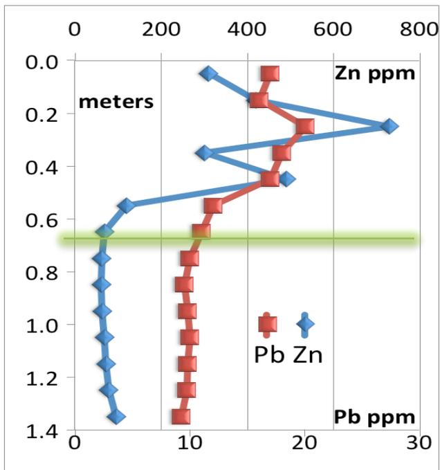
Figure 5. Zn and Pb results in the shallow pit sampled at 10 cm intervals. The position of the rubble line within the sands demarcating the original pre-drilling surface is indicated in green. Note this pit does not expose mineralization penetrating the upper aeolian sand layer only to the calcrete horizon.
