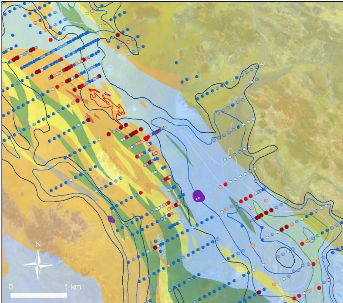
**Figure 8. Combined model used for final follow-up target selection.** This comprises subsurface geology, palaeotopography at the unconformity surface (blue lines) and calculated Skorpion index from the overburden geochemical results (coloured dots Blue low ranking to red high ranking). The >1% Zn contour of the Skorpion ore body is outlined in red. (Schaefer, 2008).
