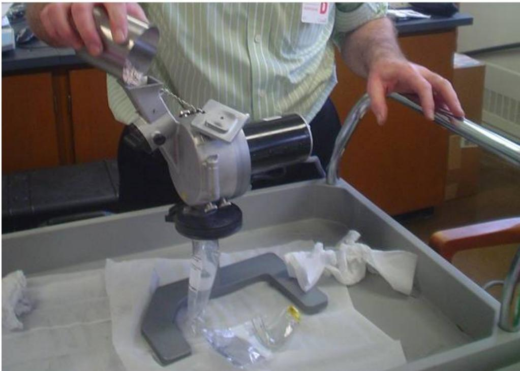
**Fig. 8.4.2. Loading the mill; note the collection bag below**
