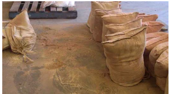
Figure 1- Dry samples received by the laboratory in calico bags may split and leak drill cuttings from one sample to the next during shipment. Spilled material is evident by the footprints on the floor.
