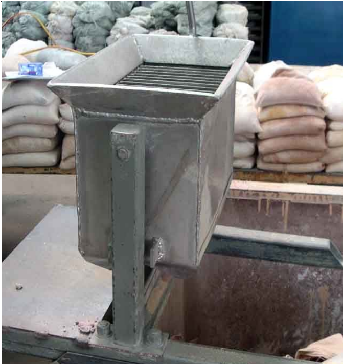
Figure 2 – Splitter used to reduce oversized samples to 3 kg before pulverizing. Samples are typically split without pre-treatment by crushing and homogenization. The excess sample is discarded.
