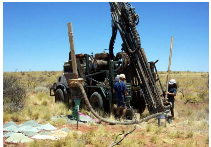
Figure 5: RAB rig showing manual rod handling and minimal site preparation. The operator has switched to hammer drilling on account of quite fresh bedrock unexpectedly encountered beneath only shallow cover (1m) and minimal oxidized profile (2-3m). Photo courtesy of Leon Marsh.
