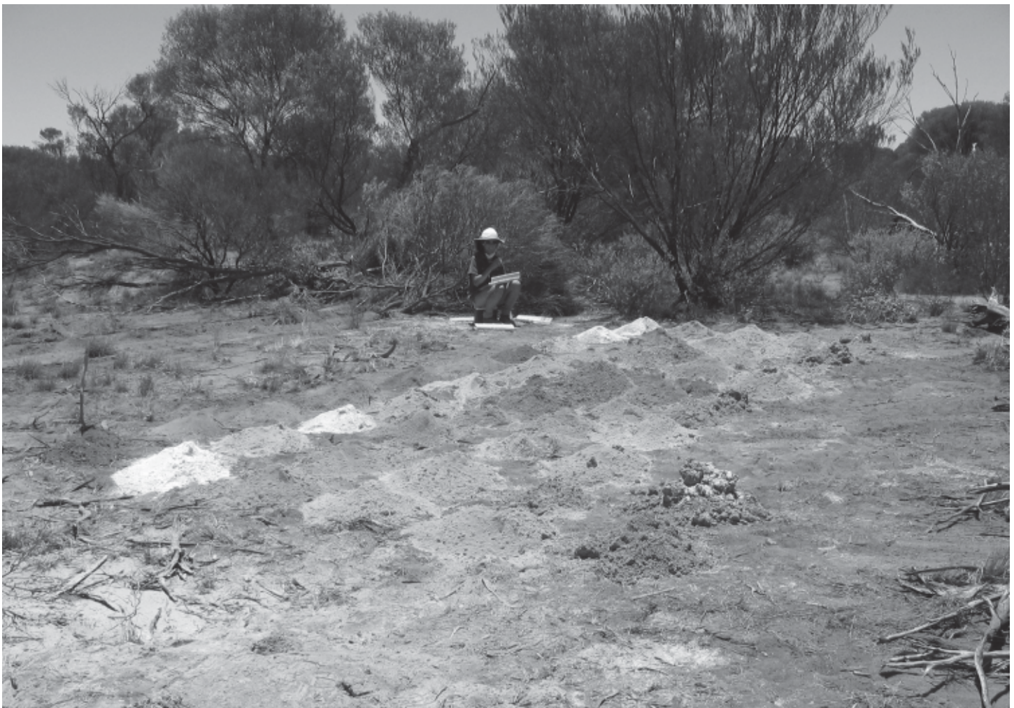
Figure 6: Photograph of RAB spoil with geologist logging. Top of hole marked by stake at centre left. Spoil piles each representing 1 meter of drilling in rows of 10. Profile shows about 8 meters of cover underlain by leached upper saprolite (white, red and purple colours) then sharp change at 39-40 meters to lower saprolite (yellow-brown-green colours). Last sample at 41-42 meters is wet and contains some fresh mafic chips. A decision is required by the geologist on a switch to hammer drilling to penetrate fresh rock if water flow can be contained so as to ensure a sample of adequate quality.
