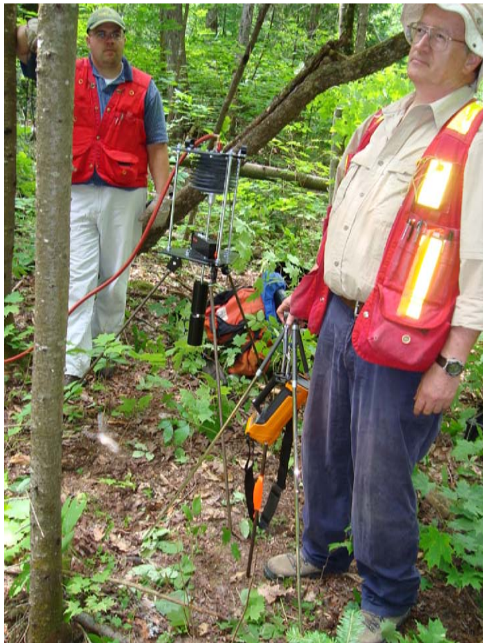
Figure 5. Brad Harvey (left) and Ken Ford (right), Geological Survey of Canada, making soil gas radon measurements at a Tri-national project site near Pembroke, Ontario. (Photo: Inez Kettles, GSC)
