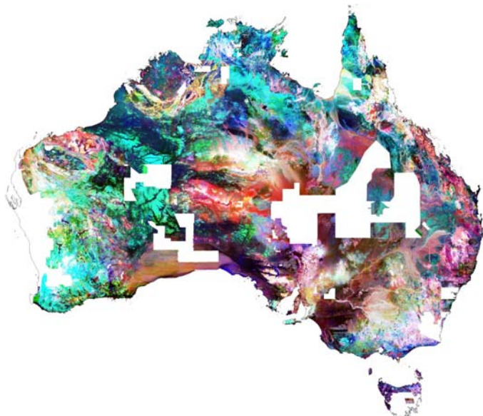
Figure 5. Ternary image of potassium (red), uranium (blue) and thorium (green) radioelement estimates across Australia after levelling surveys with AWAGS data.
