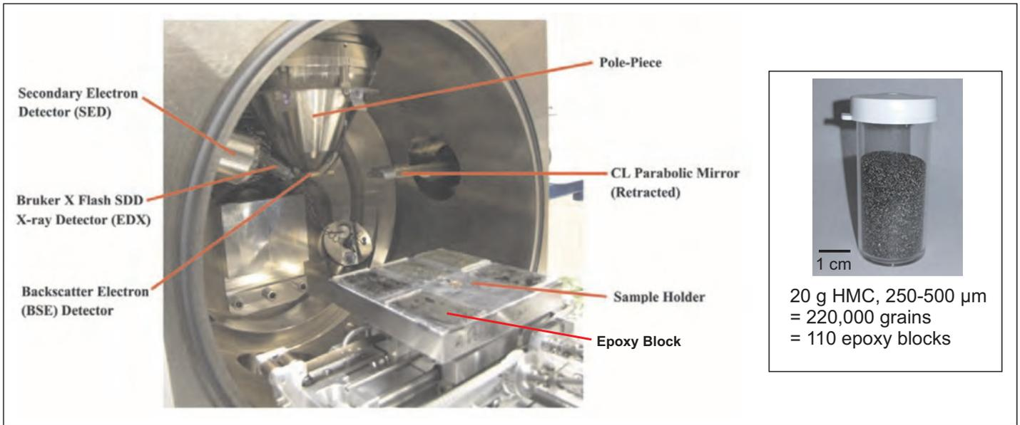
Figure 4. Grain capacity of an automated mineral analyzer. Each epoxy block in the sample tray will hold  $\sim 2,000$  grains of 250-500  $\mu\text{m}$  (medium sand) size or 8,000 grains of 125-250  $\mu\text{m}$  (fine sand) size. However, a typical 10 kg till sample contains  $\sim 20$  g of heavy minerals of each size and each gram contains 11,000 or 88,000 mineral grains, respectively, for a total of 220,000 or 1,760,000 grains requiring 110 or 220 epoxy blocks to be analyzed completely.
