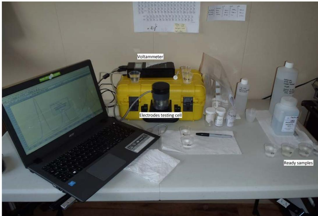
*Figure 3. Photograph from 2016 study showing the portable voltammeter set-up. The instrument is resting on top of the yellow case, and the cell containing the test electrodes and the water sample rest on a holder just above the case handle. Laptop is not required for voltammeter operation.*
