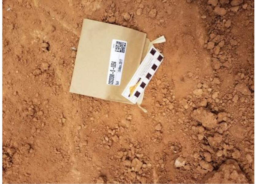
Figure 4. Soil sampling showing the field printed labels and data matrix bar-code for scanning the sample identifier into the mobile application.
