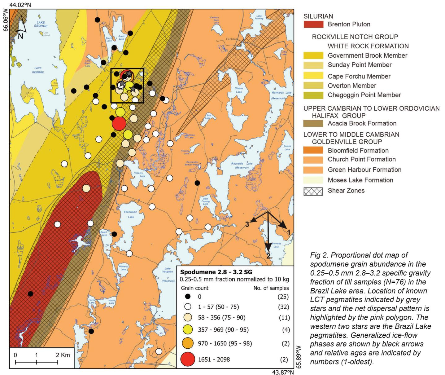
Fig 2. Proportional dot map of spodumene grain abundance in the 0.25–0.5 mm 2.8–3.2 specific gravity fraction of till samples (N=76) in the Brazil Lake area. Location of known LCT pegmatites indicated by grey stars and the net dispersal pattern is highlighted by the pink polygon. The western two stars are the Brazil Lake pegmatites. Generalized ice-flow phases are shown by black arrows and relative ages are indicated by numbers (1-oldest).
