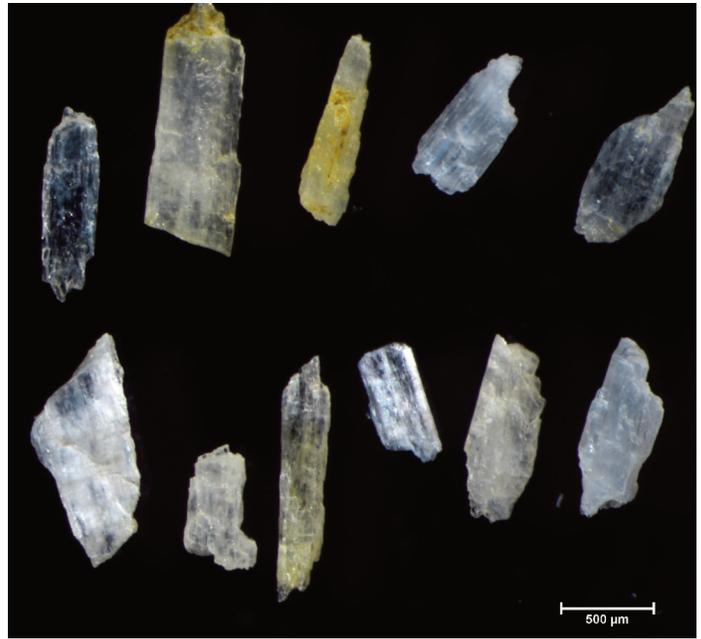
Fig. 5. Colour photograph of spodumene grains from a bedrock sample of the North Brazil Lake pegmatite. Photograph taken by Overburden Drilling Management Ltd).
