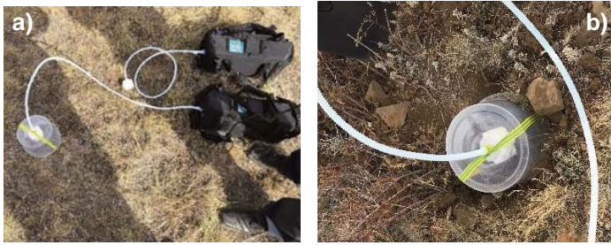
Fig. 3. Near-surface air sampling (a) 1 cm above undisturbed surface and (b) after removing the top 5 to 15 cm layer across an area of ca. ~20 cm in diameter. White tubing transports air collected from the bucket probe to the mercury analyzer inside the black bag.
