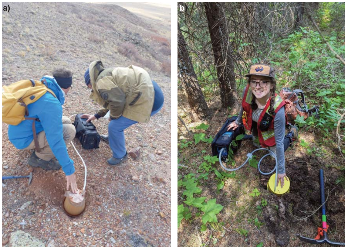
Fig. 6. Sampling air mercury 1 cm above ground using a bucket probe after removing the top 5 to 15 cm layer across a sampling area of ~20 cm in diameter. a) Central Kazakhstan, 2022. b) Central British Columbia, Canada, 2023.
