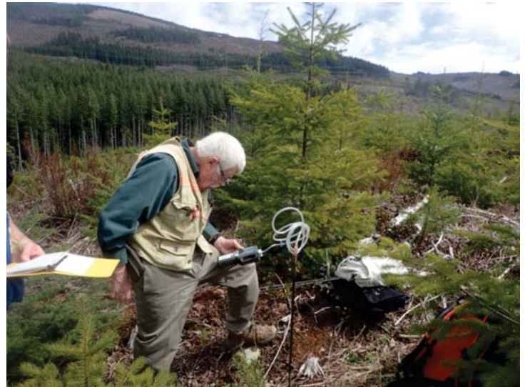
Fig. 12. Collecting soil gas for CO 2 , O 2 and CH 4 analysis using the CO 2 Meter GasLab® Pro Multi-Gas CM 1000 Data Logger on the Anita property.
