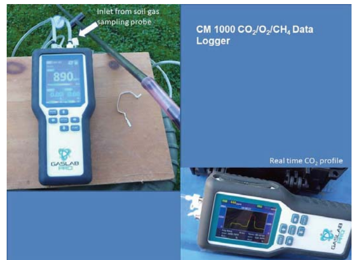
Fig. 3. Display and port hoses on the CO2Meter GasLab® Pro Multi Gas Sampling CM 1000 Data Logger.
