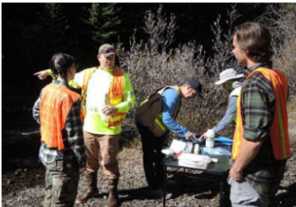
Figure 4: Garth Graham demonstrates clean procedures for water sample collection, water pH and alkalinity measurements, sample filtering and acidification.
