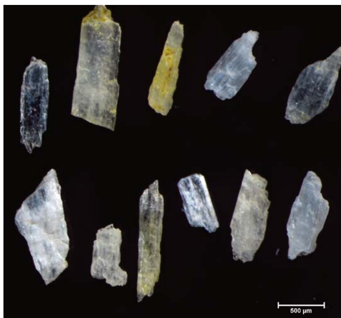
Fig. 5. Colour photograph of spodumene grains from a bedrock sample of the North Brazil Lake pegmatite. Photograph taken by Overburden Drilling Management Ltd).
