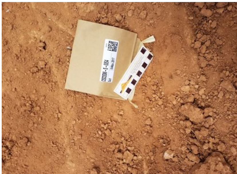
Figure 4. Soil sampling showing the field printed labels and data matrix bar-code for scanning the sample identifier into the mobile application.
