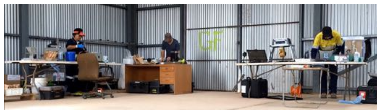
Figure 5. The portable laboratory at Coompana. From left to right, riffle splitter, crusher and mill on one table, pellet press on the old desk, the fpXRF and ASD (inside cardboard box, far right) on the other table.
