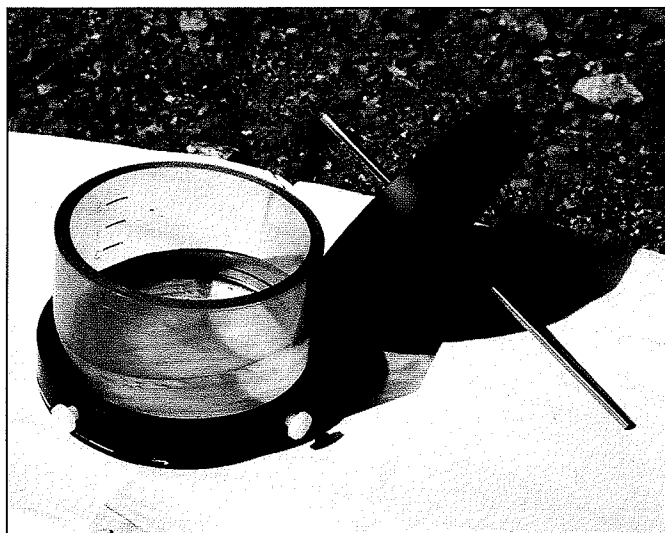
The USGS-designed ion collector electrode for testing the electrogeochemical sampling method, CHIM, and a variation thereof, APLOCHIM.
