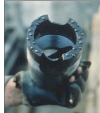
Bit with tungsten carbide bit
