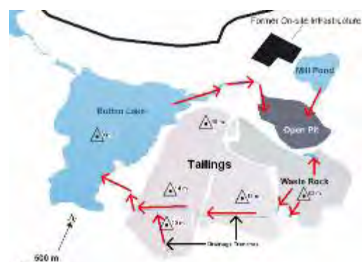
Fig. 1. Map of Ruttan mine site showing the drainage trenches in the tailings and flow direction of drainage water.
