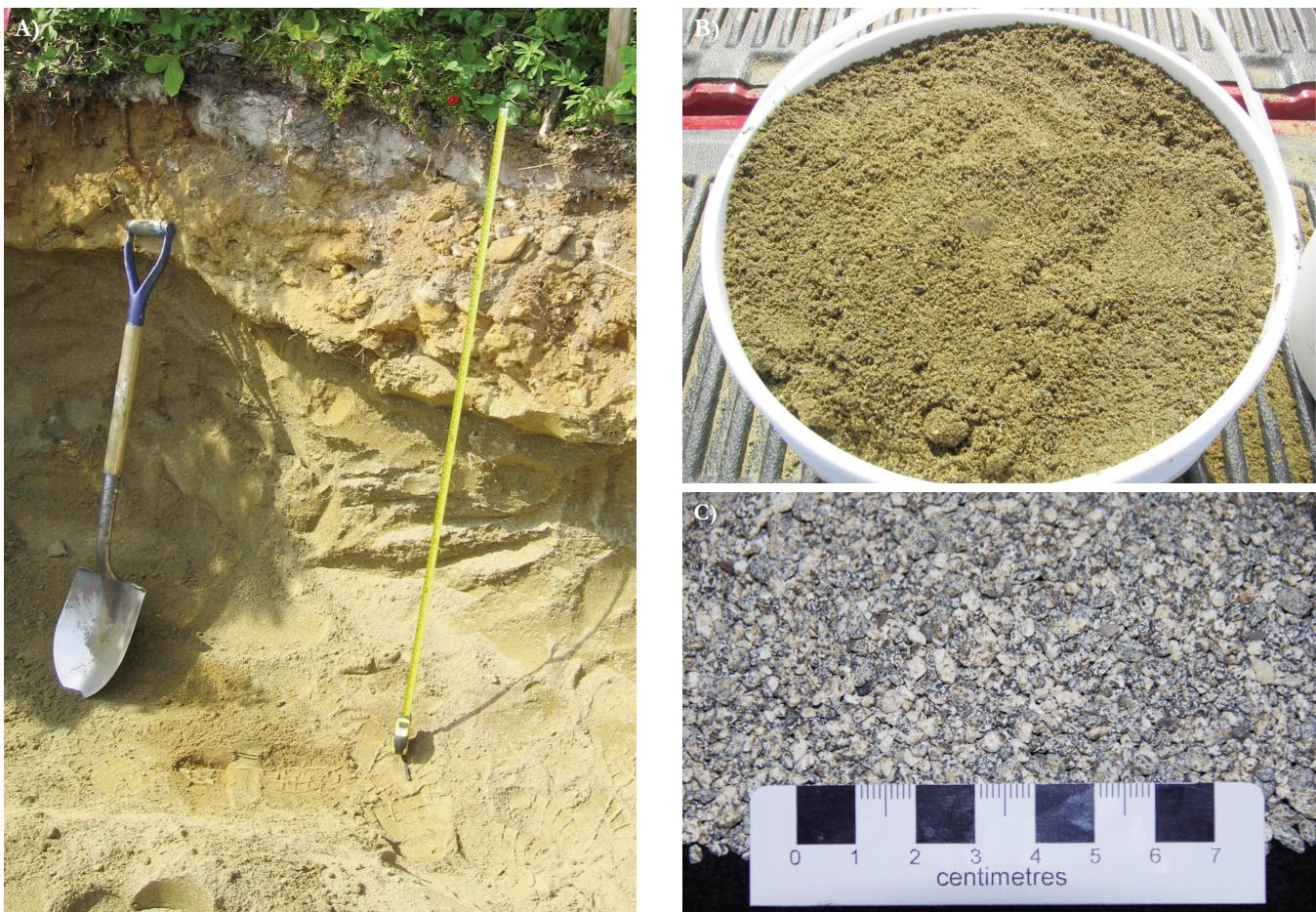
**Fig. 8.** **A)** Sample site of the unconsolidated weathered Silurian-Devonian granite (grus) used for GSC blank heavy mineral samples. **B)** Close-up view of the blank sample material. **C)** Close-up view of the 2–4 mm fraction of the blank material.
