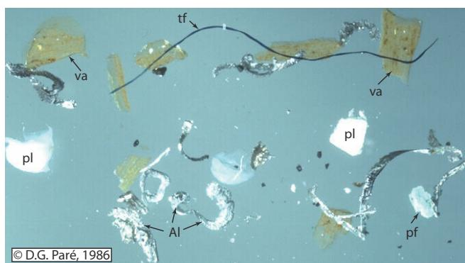
**Fig. 2.** Examples of contamination in heavy mineral concentrates including plastic from vial cover (pl), textile fibre (tf), aluminum shavings (Al), varnish flakes with traces of wood fibre (va), and paint flakes (pf); photographs from D.G. Paré, Consorminex Incorporated, Gatineau, QC ([www.consorminex.com](http://www.consorminex.com)).
