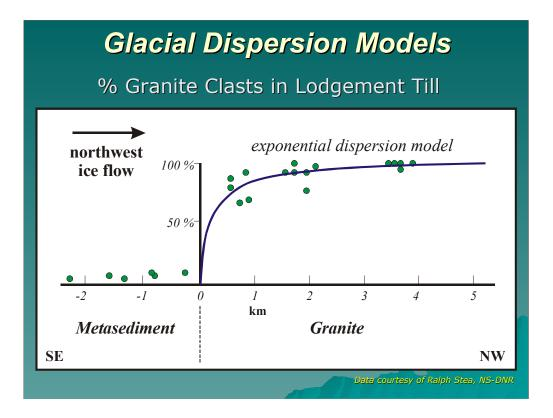
This example illustrates how the concentrations of granite clasts in the till increase across a meta-sedimentary rock-granite contact. These data have been regressed using an exponential dispersion model.
