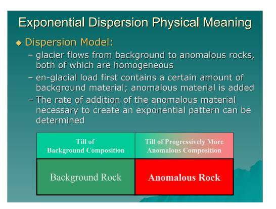
To illustrate my conclusions, consider a simple model where the initial en-glacial load should contains only background material. After flowing past the contact onto an anomalous rock, the anomalous lithology is eroded and added to the en-glacial load, eventually being re-deposited as till.
