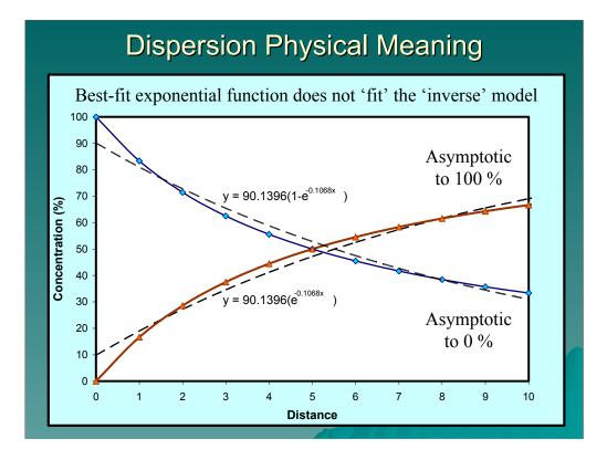
This is a graphical comparison of the inverse function and the 'best fit' exponential function. The differences between these functions are clear.
