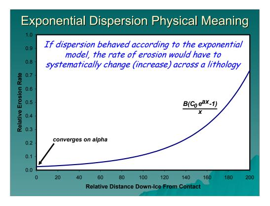
The amount of material that must be added to the en-glacial load to create an exponential dispersion pattern is presented in this scale independent graph. Clearly, the erosion rate must increase significantly with distance (provided topographical variations are absent) to produce the exponential pattern.
