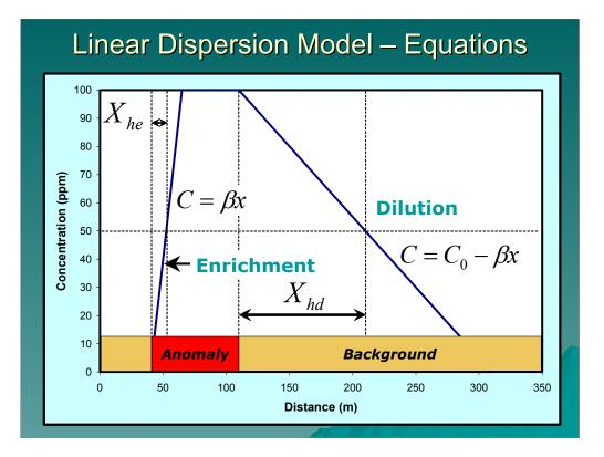
Like the exponential model, the linear dispersion model also has corresponding equations describing how concentrations increase and decrease down-ice from a geological contact.
