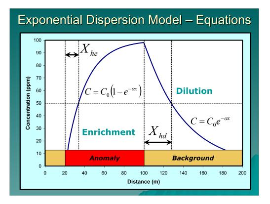
Numerical equations involving a negative exponential function have historically been used to describe the dilution and enrichment of the concentrations of anomalous and background material in the till.
