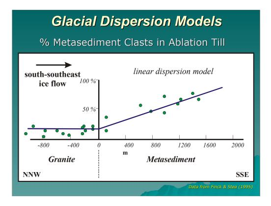
Similarly, this example illustrates how the concentrations of metasediment clasts in the till increase across a granite-meta-sedimentary rock contact. These data have been regressed using a linear dispersion model.
